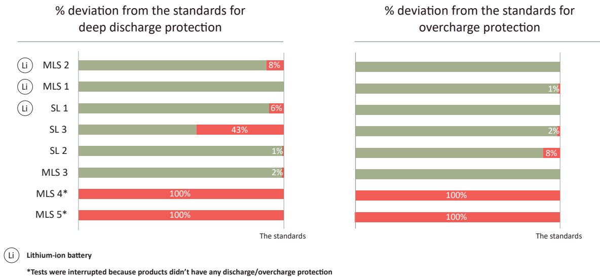
Figure 9 : Deviation from Lighting Global Quality Standards for battery protection
