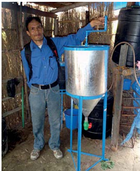
Small struvite reactor (source: Eawag)
