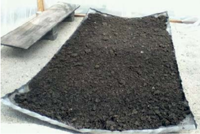
Fecal sludge in transition to granular fuel inside solar greenhouse. Source: www.waste-enterprisers.com
