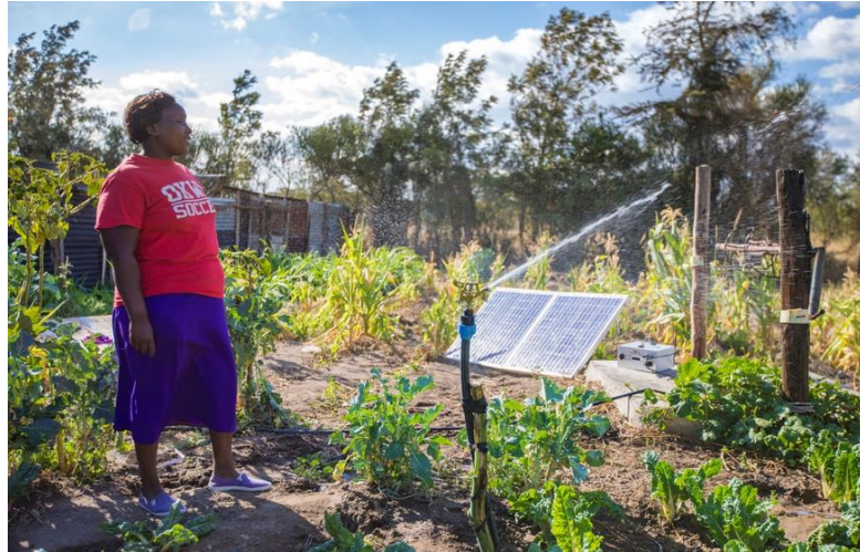
SunCulture's pump with sprinklers, Credit: SunCulture
